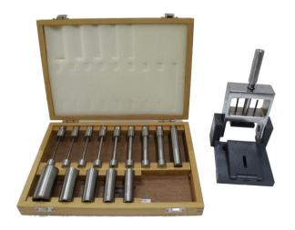
This test is carried out by bending the coated panel around mandrels of different diameters until damage occurs. Max. panel size: 70mm width and 0.8mm thick.
