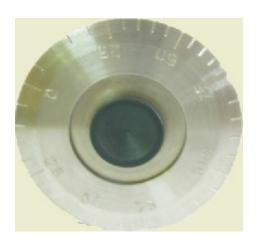
A stainless steel precision gauge to check wet film. A wheel machined with an eccentric central rim calibrated to increasing gap is rolled across the paint. The contact point on the rim indicates the film thickness.
