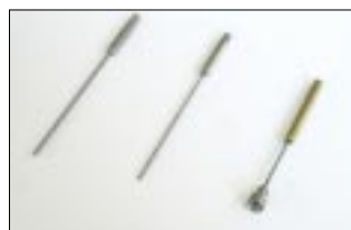
Needles 1.13 mm, 1 mm, final setting.
