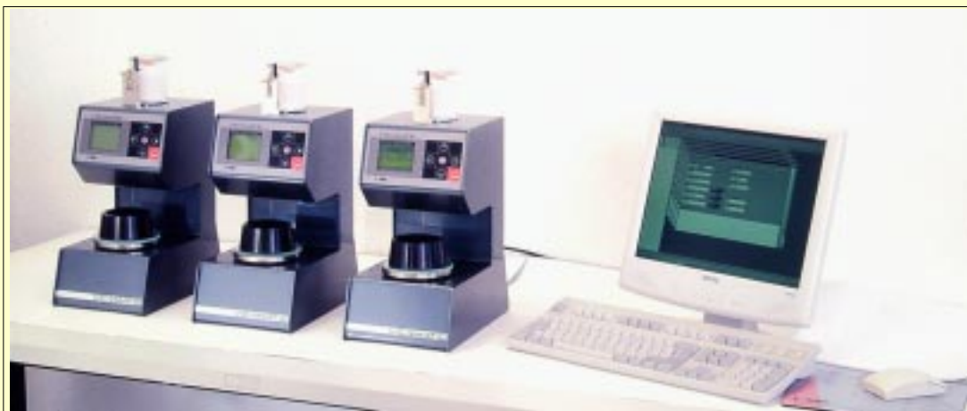
Schematic view of a multiple Vicat testing systems (up to 16) connected to PC.
