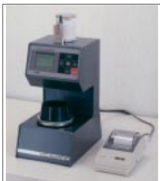
VICAMATIC connected to serial printer (see accessories).
