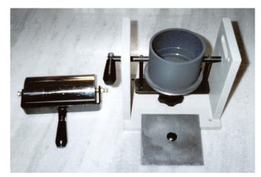
'CI' Cobb Tester is a sturdy and precise instrument with non-corrosive all aluminium powder coated body. The instrument is provided with a marker to indicate the exact level of water required, also ensuring uniformity of water level over the samples. A gasketed clamping arrangement for the sample on the underside of the cylinder. Tilting provision has been provided for easy draining of water after test, the cylinder gets locked on turning by180° and the knob can be used as a handle.
